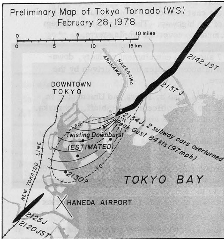
Figure 7.8 Schematic map of Tokyo tornado preceded by an estimated twisting downburst, 2 to 4 miles wide.
